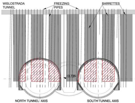
Figure 12. Scheme of the freezing pipes to be shortened under WS for the further cut of the barrettes.
