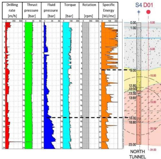
**Figure 1. Soil stratigraphy obtained from borehole S4 compared with drilling parameters of DPR test D01 after the filling with lean mix concrete and grouting operations.**
