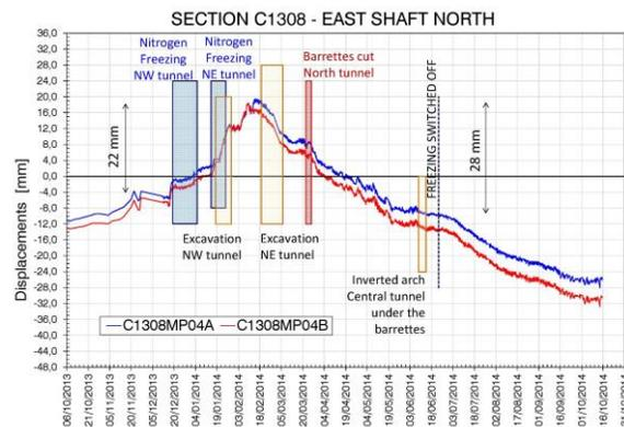
Figure 14. Wislostrada displacement diagrams.
