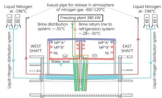
Figure 6. Freezing plants installed on site for direct (Liquid Nitrogen) and indirect (brine) method.
