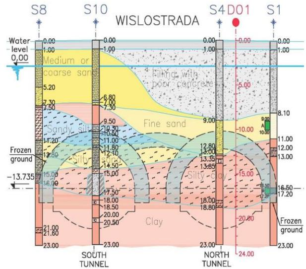
**Figure 2. Soil stratigraphy at the West shaft with frozen ground arches around the tunnels.**
