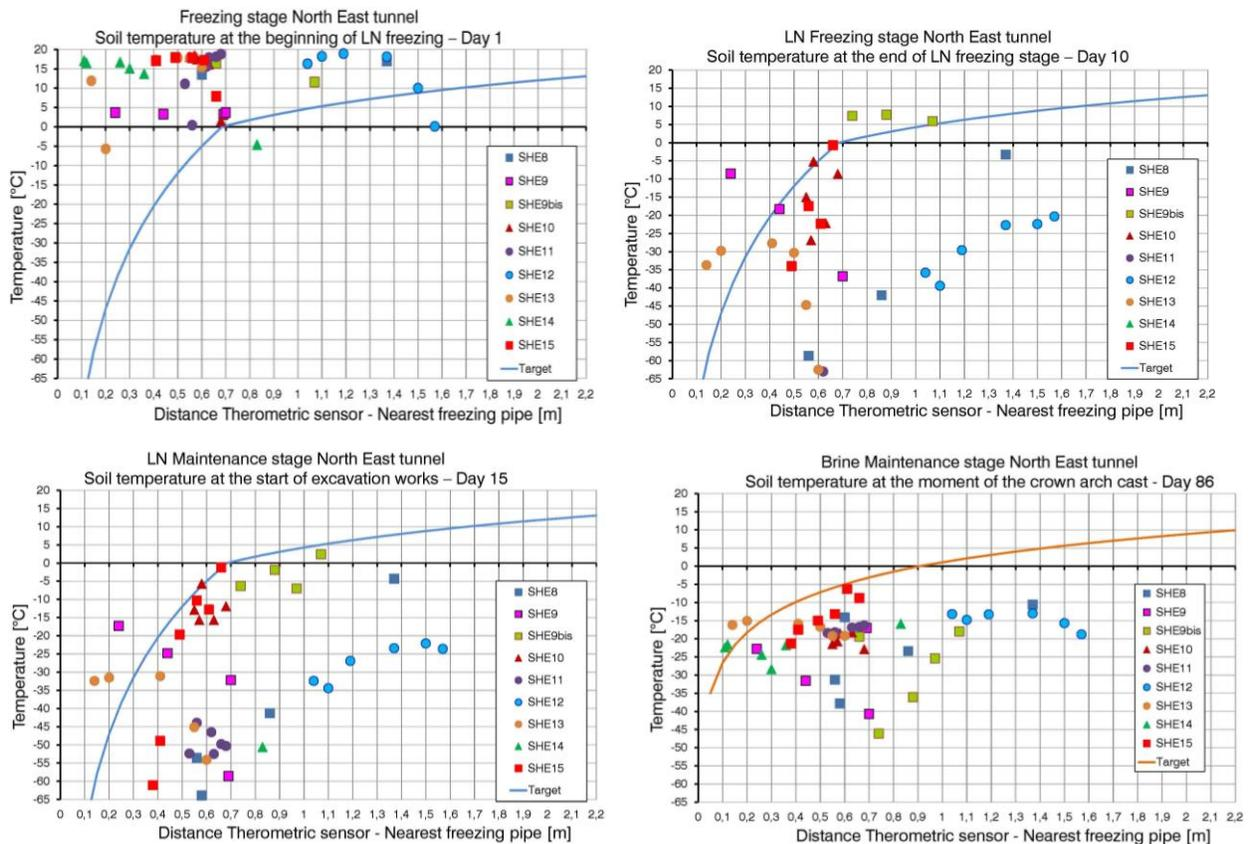
**Figure 9. Ground thermometric vs. sensor distance from the freezing pipe at different times of the works.**
