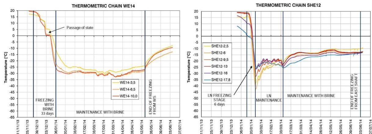
Figure 8. Ground temperature evolution in thermometric chains WE14 and SHE12.
