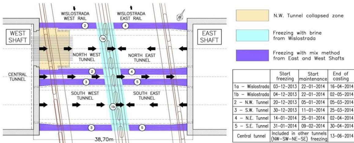
Figure 7. Ground freezing and excavation phases layout.
