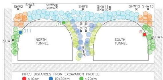
**Figure 4. The effective position of freezing and thermometric pipes surveyed with the Reflex Maxibor II system at a distance of 10m from the front wall of the West shaft.**
