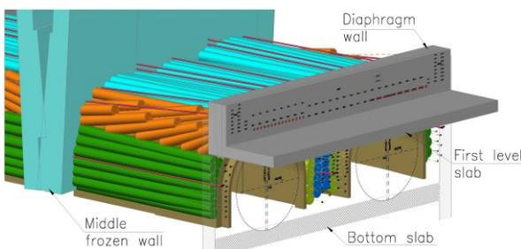
**Figure 3. Freezing pipes geometry. In the background the vertical frozen walls installed from Wislostrada and in foreground the pipes installed from the West shaft.**
