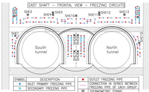
Figure 5. Freezing pipes circuits and thermometric strings layout in East shaft.
